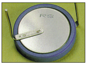
Lithium-ion coin cell battery tab
