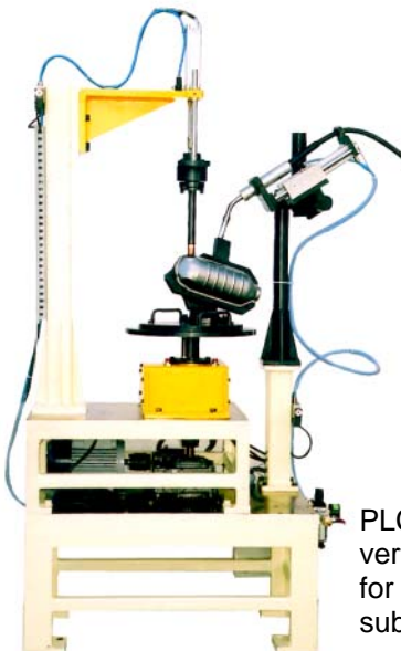
Horizontal SPM for circular welding of exhaust converter.
