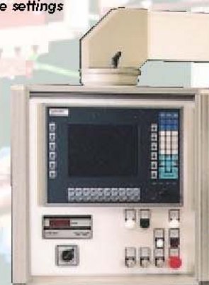
Figure 2: Typical advanced programmable weld and force settings
