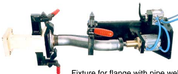
Fixture for flange with pipe welding suitable for horizontal SPM.
