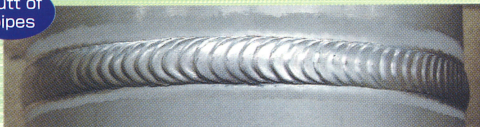
Pulsed current 200A, Base current 20A, Pulse frequency 2Hz AC frequency: 150Hz, Welding speed: 20cm/minute, Plate thickness: 4mm (A6062)
