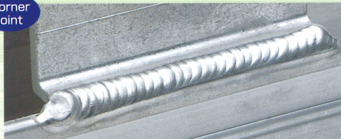
Welding current: 130A, AC frequency: 150Hz Welding speed: 25cm/minute, Plate thickness: 3mm (A6063 + Casting)
