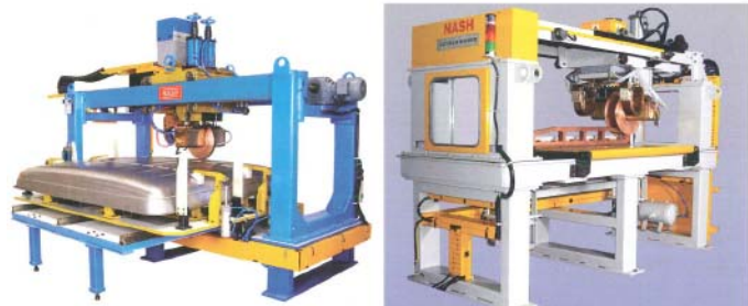
Application: Twin Lap Seam Welding for Front and Rear Roof Joining of HCV Cab
